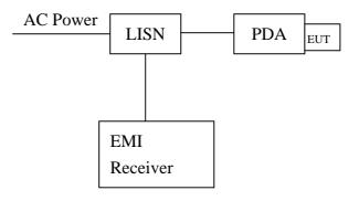
The EUT are connected to the main power through a line impedance stabilization network (LISN). This provides a 50 ohm/50uH coupling impedance for the measuring equipment. The peripheral devices are also connected to the main power through a LISN that provides a 500hm/50uH coupling impedance with 500hm termination.
