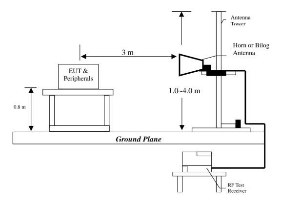
Radiated emissions were invested cover the frequency range from 30MHz to 1000MHz using a receiver RBW of 120kHz record QP reading, and the frequency over 1GHz using a spectrum analyzer RBW of 1MHz and 10Hz VBW record Average reading. (15.209 paragraph), the Peak reading (1MHz RBW/VBW) recorded also on the report.
