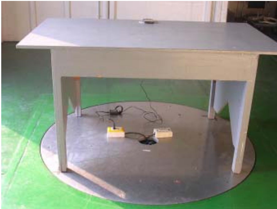
Photo 2: Radiated Emission Test Set-up
