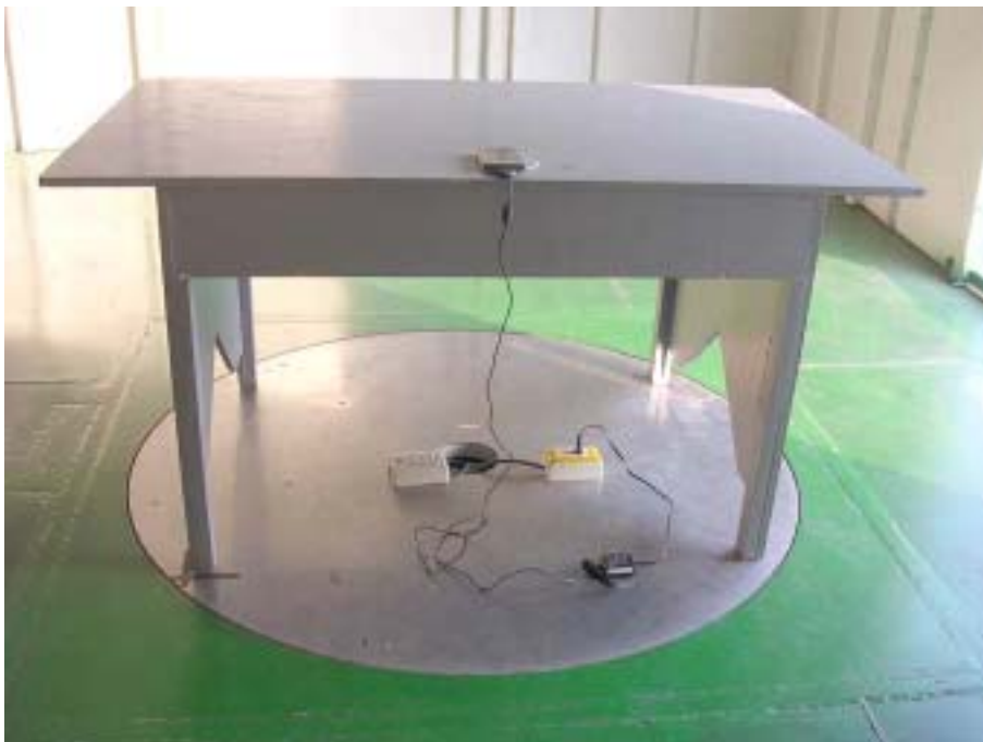
Photo 2: Radiated Emission Test Set-up
