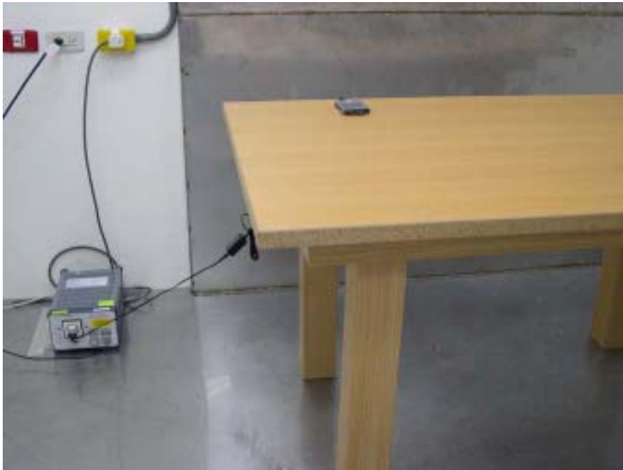
Photo 2: Conducted Emission Test Set-up
