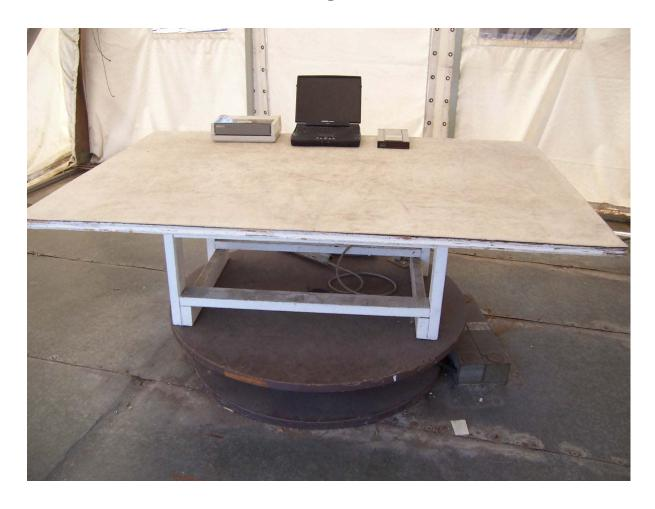
Radiated Emissions Test Setup
