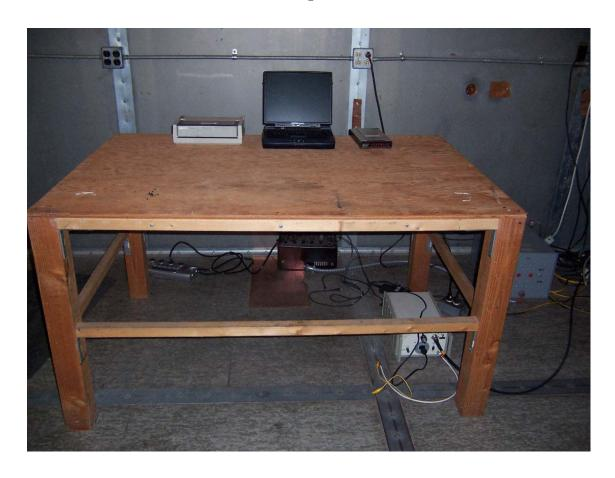
Line Conducted Emissions Test Setup
