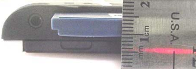
9 mm Spacing from CF Card to Front Side of Host PDA
