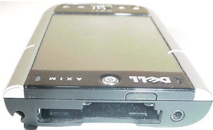
CF Card Slot - Top End of PDA (Compact Flash Card Removed)
