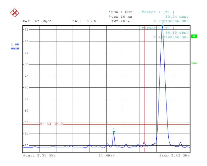
Comment: Band-edge test at low channel Comment: Average detector  $F2{=}2390\,\text{MHz}$
