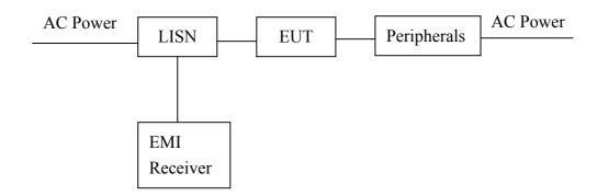
The EUT are connected to the main power through a line impedance stabilization network (LISN). This provides a 50 ohm/50uH coupling impedance for the measuring equipment. The peripheral devices are also connected to the main power through a LISN that provides a 500hm/50uH coupling impedance with 500hm termination.
