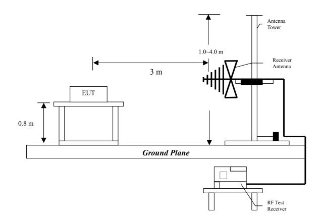
Radiated emissions were invested cover the frequency range from 30MHz to 1000MHz using a receiver RBW of 120kHz record QP reading, and the frequency over 1GHz using a spectrum analyzer RBW of 1MHz and 10Hz VBW record Average reading. (15.209 paragraph), the Peak reading (1MHz RBW/VBW) recorded also on the report.
