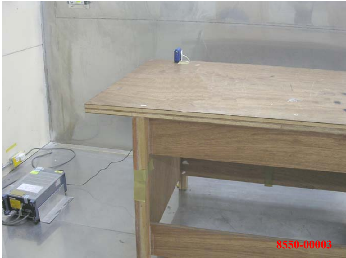
Photo 1: Conducted Emission Test Set-up
