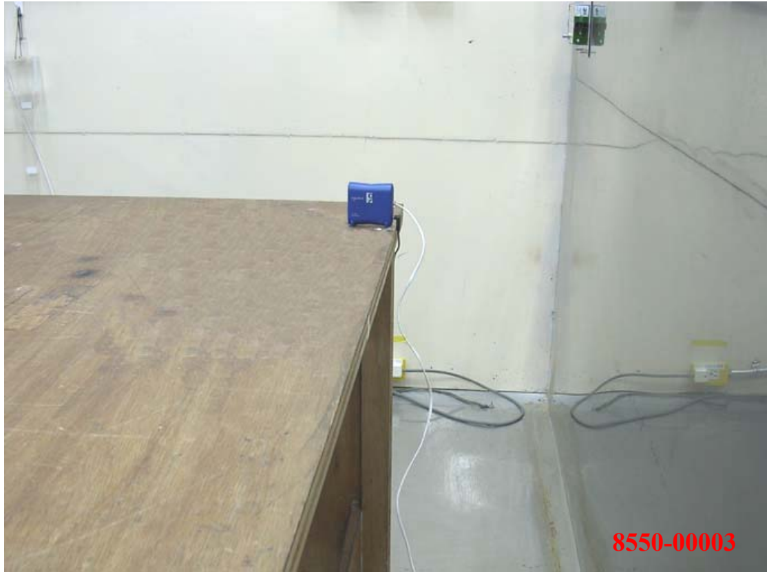
Photo 2: Conducted Emission Test Set-up
