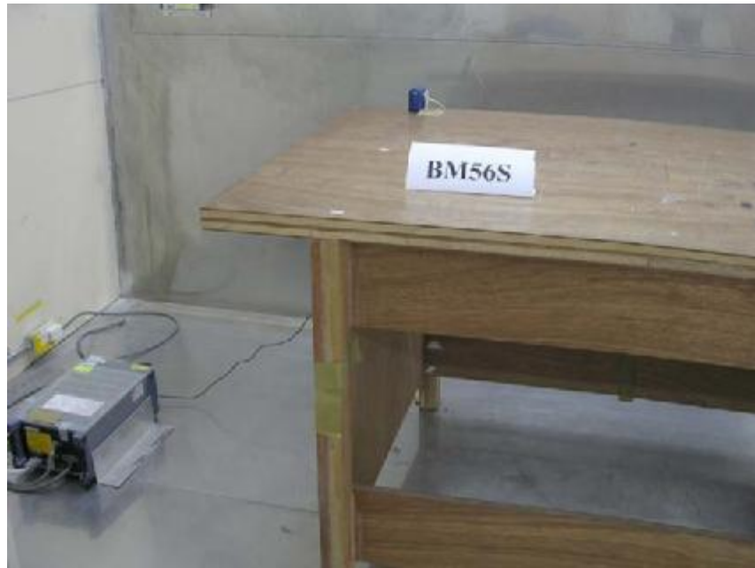
Photo 2: Conducted Emission Test Set-up
