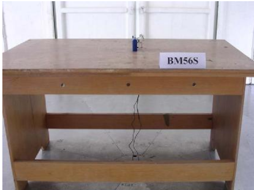
Photo 2: Radiated Emission Test Set-up
