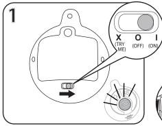
Move the switch on the back of the controller to the ON (1) position. The light on the center button of the remote will flash.
