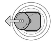
If you crash, immediately press and hold the landing / emergency stop button for two seconds.
