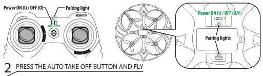
Place the drone on a flat surface. Stand 3 feet from the drone and press the auto take off button to launch it. Then, use the joysticks to maneuver it.
