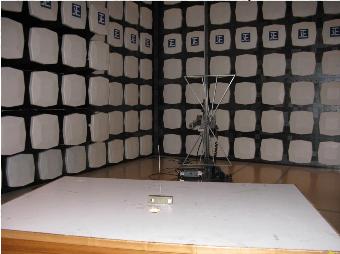
Measurement of Radiated Emission Test Set Up
