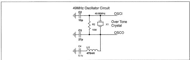
Note: There are different values of C2, C3 and L1 for 27MHz, 40MHz and 49MHz. User must use these values correctly, otherwise it possibly casues oscillator circuit malfunction.
