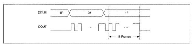
The GPRC206A1 is able to receive serial bit-stream data transmitted from GPRC205A1 and decode the data fields as 5-bits data output. Any signal on DIN pin will activate GPRC206A1 to decode the incoming data. When GPRC206A1 receives two
