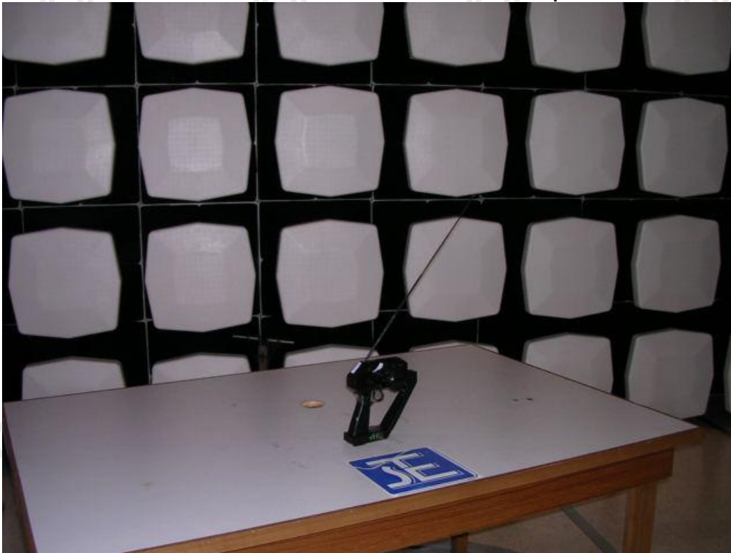
Measurement of Radiated Emission Test Set Up
