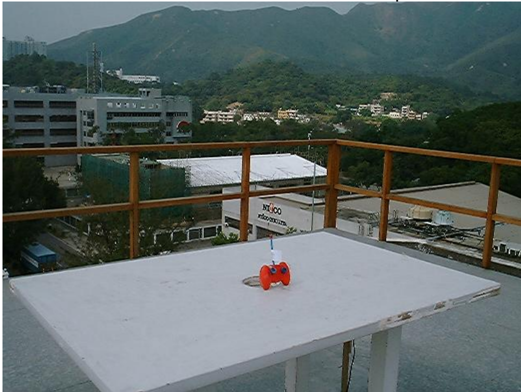
Measurement of Radiated Emission Test Set Up
