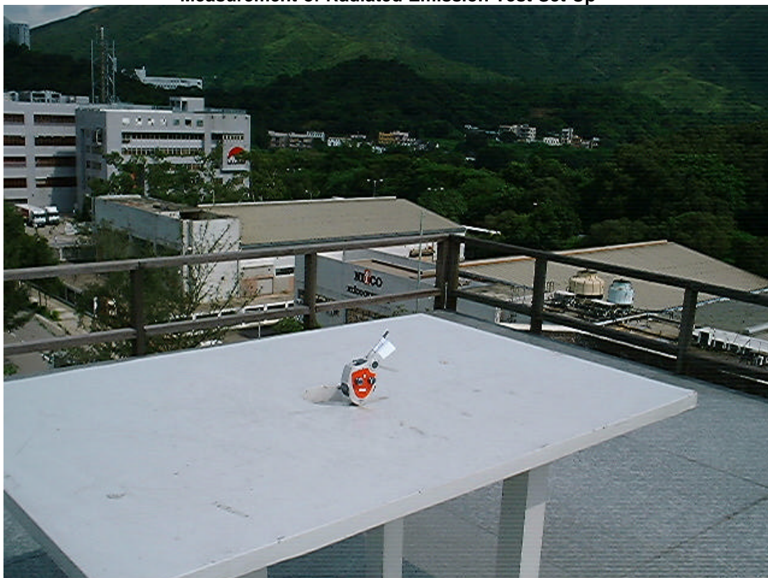
Measurement of Radiated Emission Test Set Up
