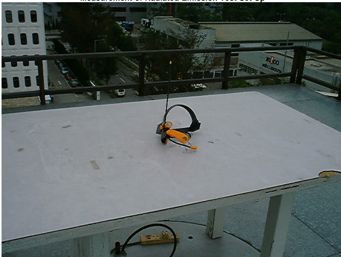
Measurement of Radiated Emission Test Set Up
