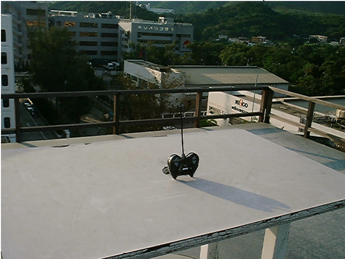
Measurement of Radiated Emission Test Set Up
