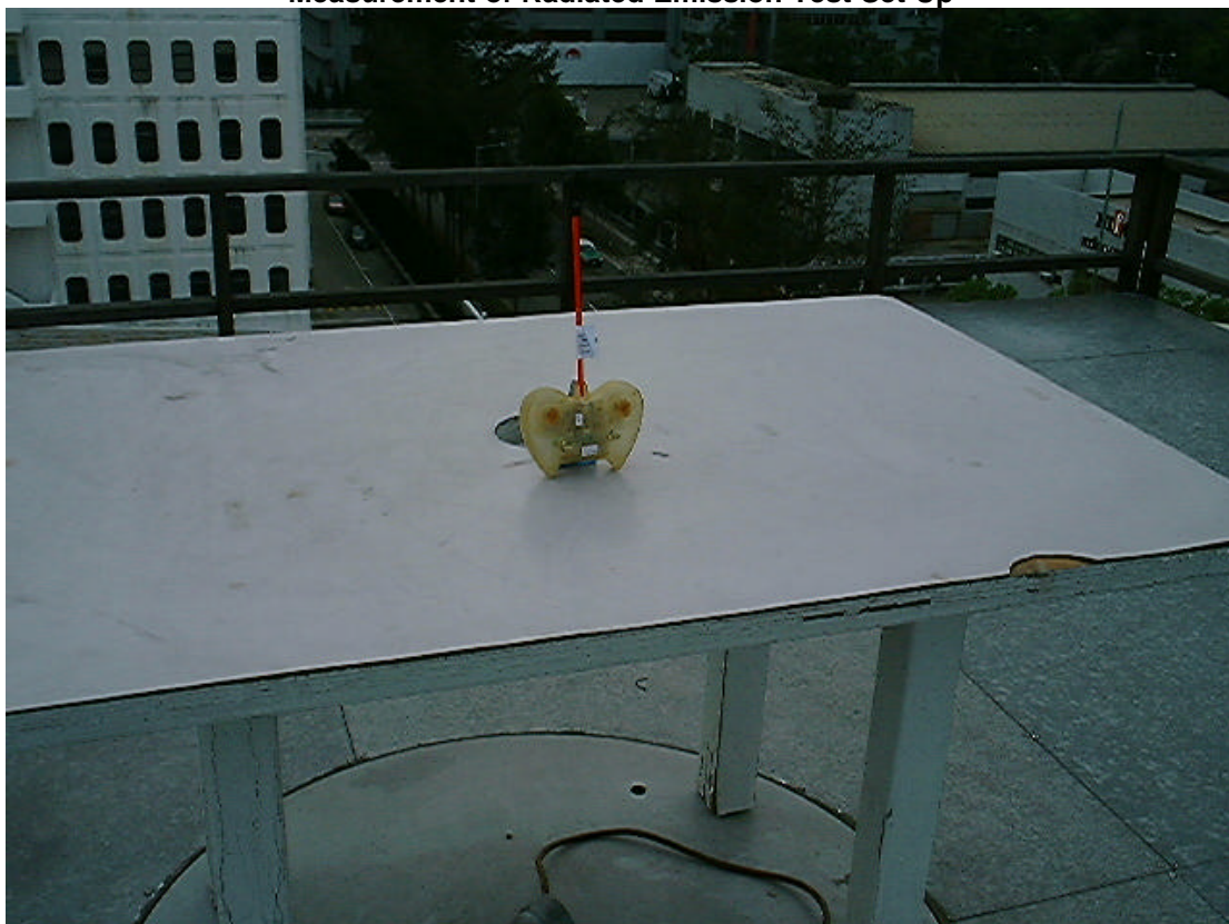
Measurement of Radiated Emission Test Set Up
