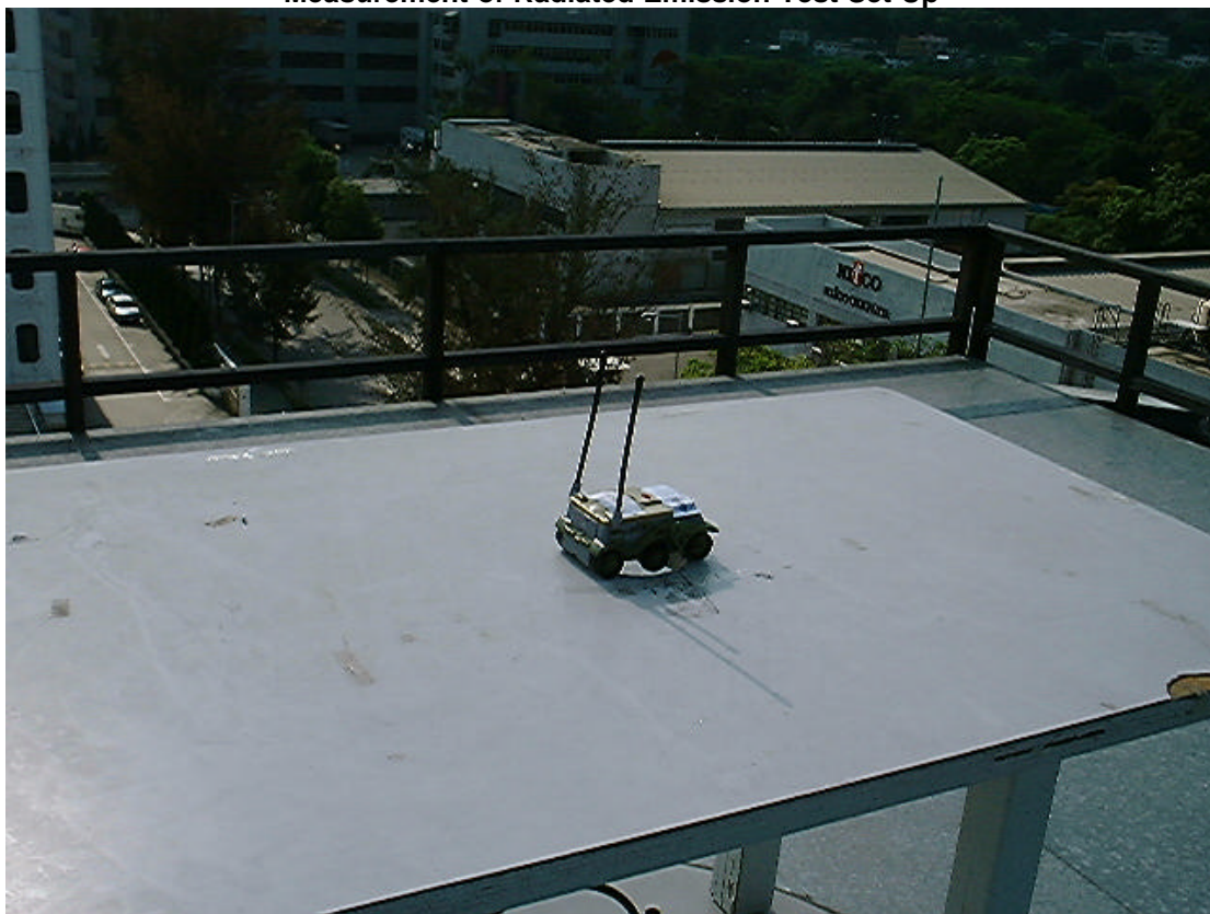
Measurement of Radiated Emission Test Set Up
