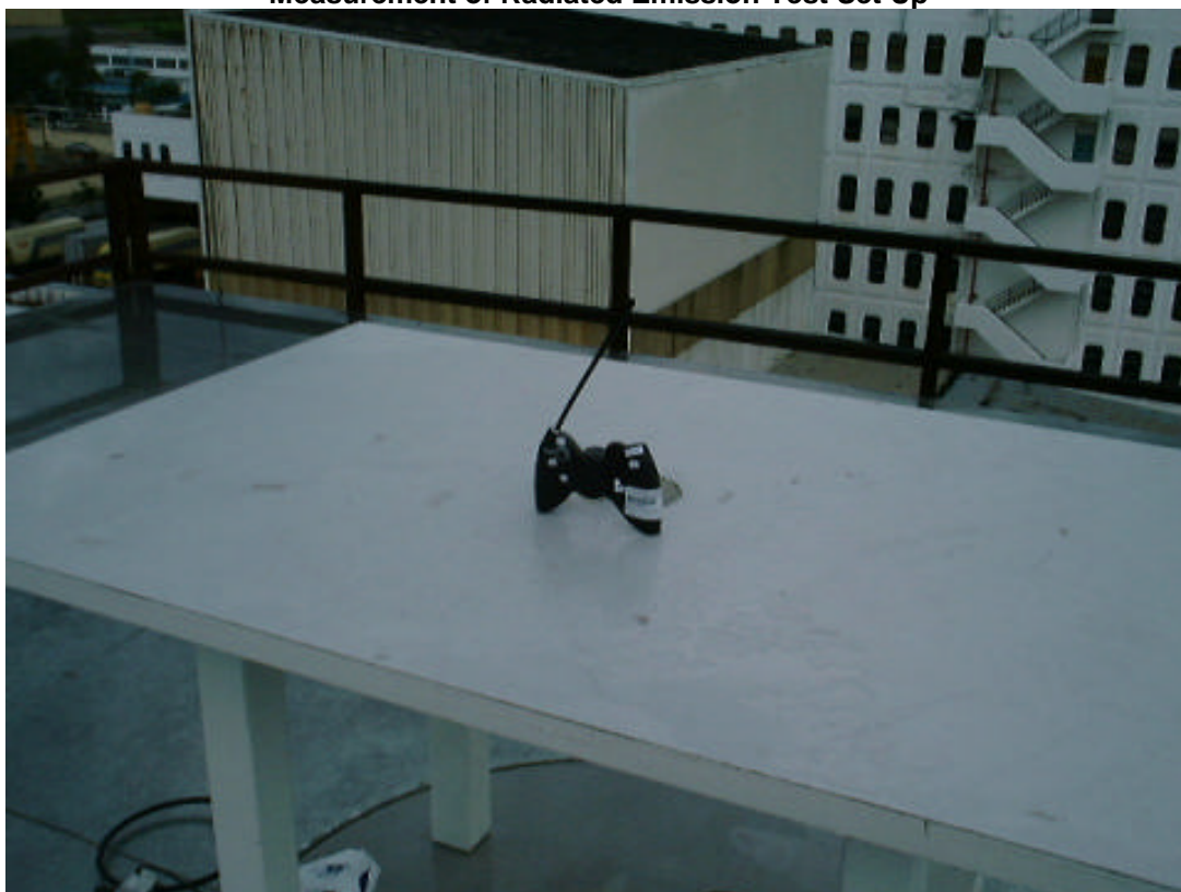
Measurement of Radiated Emission Test Set Up
