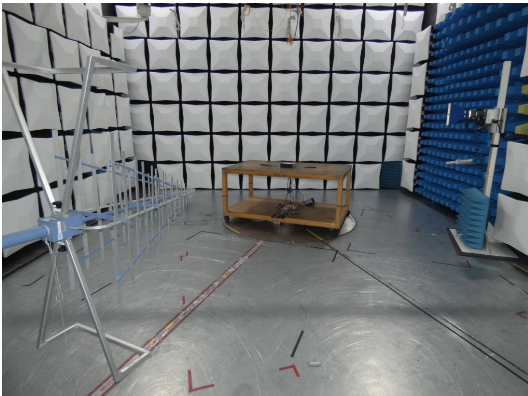
Photo 2: Test setup for radiated measurements (30 MHz - 1 GHz)
