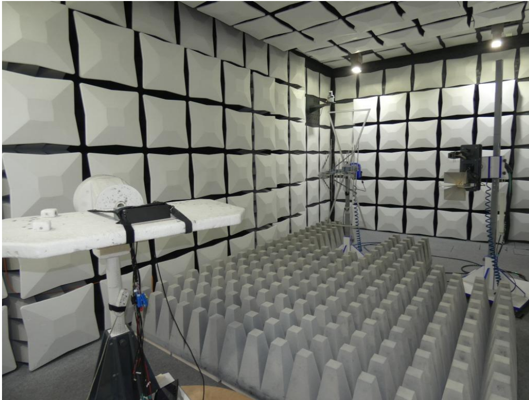
Photo 3: Test setup for radiated measurements above 1 GHz
