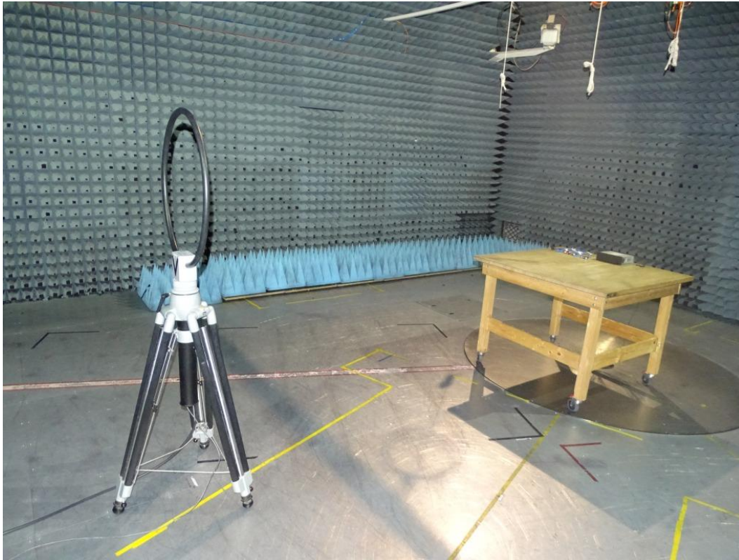
Photo 1: Test setup for radiated measurements (9 kHz - 30 MHz)
