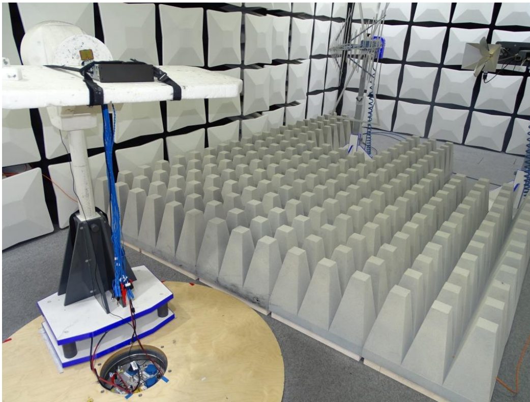
Photo 3: Test setup for radiated measurements above 1 GHz
