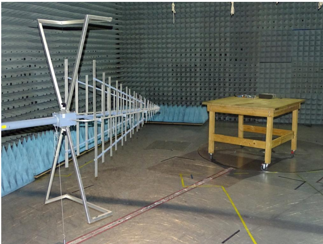
Photo 2: Test setup for radiated measurements (30 MHz - 1 GHz)
