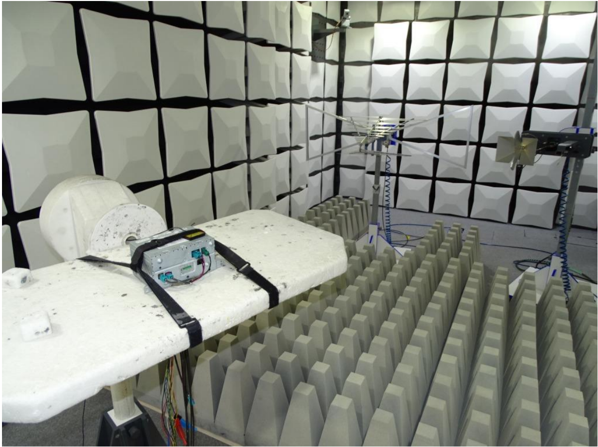
Photo 3: Test setup for radiated measurements above 1 GHz
