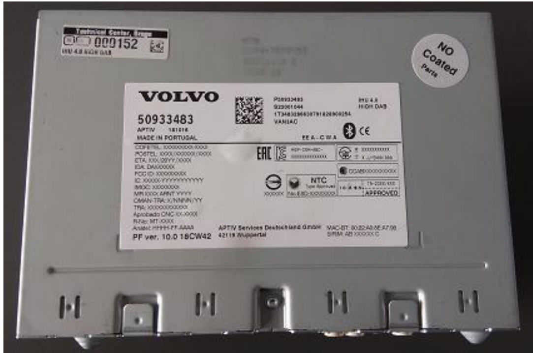
Figure 15 - IHU 4.0 Label Location (Variant: IHU 4.0 High DAB)
