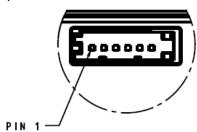
MATING INTEREFACE (HARNES CONNECTOR) TO BE USED FORD P/N: 4F1T-14489-AB TYCO P/N: 1488752-3 KEYING OPTION "C"
