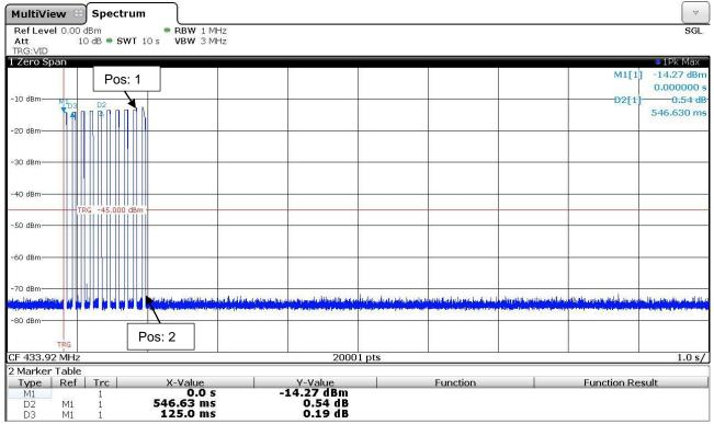
RKE (Remote Keyless Entry) - Activation of Transmission Long Single button pressed and released.
