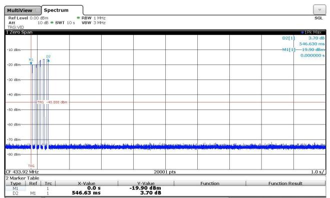
RKE (Remote Keyless Entry) - Activation of Transmission Short Single button pressed and released.
