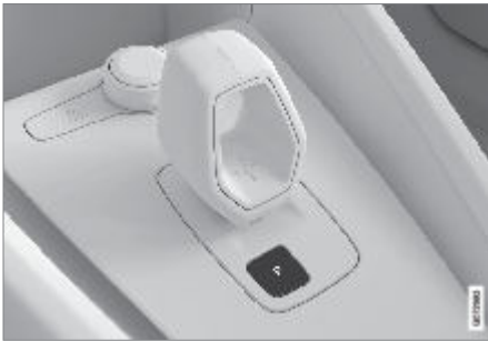
The button for the parking brake is located next to the gear selector.
