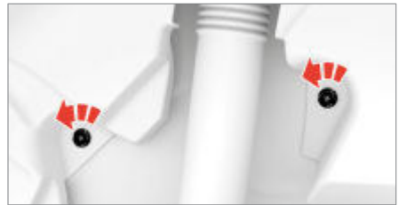
The nuts to be loosened are located on each side of the shock absorber.
