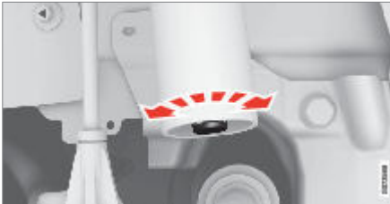
Turn the adjuster knob clockwise and anticlockwise respectively to change adjustment position.
