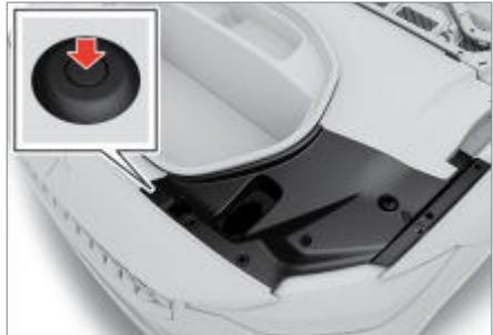
Loosen the 5 fasteners and lift up the panel.
