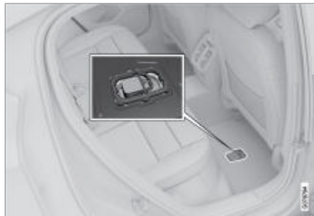
The safety switch is fitted in the floor behind the right-hand front seat.
