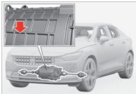
Location of punched-in serial number and model for front electric drive motor.
