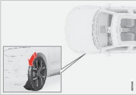
The arrow shows the tyre's direction of rotation.
