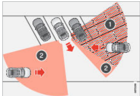
In an angled parking slot, the sensors may be completely blocked on one side.
