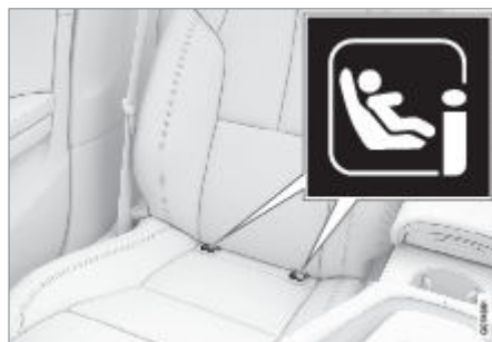
Mounting point locations for the front seat are indicated by symbols on the upholstery of the backrest.
