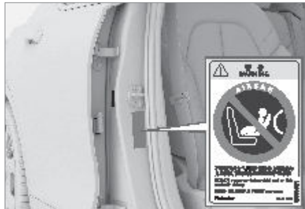
Label on the passenger side's door pillar. The label becomes visible when the passenger door is opened.
