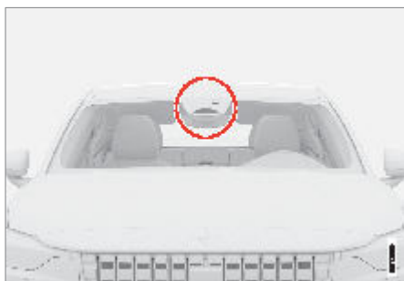
Location of the camera unit
