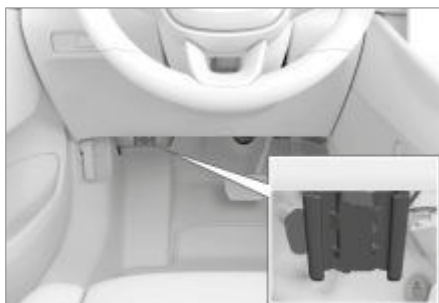
Data link connector (On-board Diagnostic, OBDII) is under the instrument panel on the driver's side.
