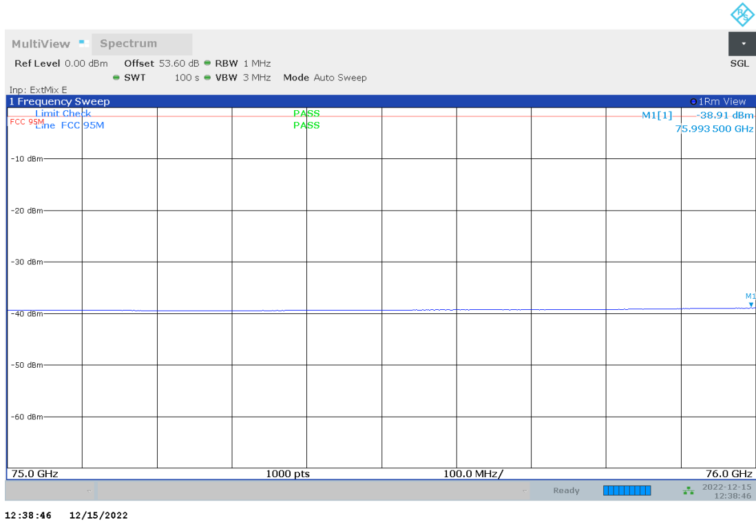
Plot no. 69: radiated emissions 75 GHz – 76 GHz, BEC low, f_{high} , Mode 1, polarization aligned with radar sensor
