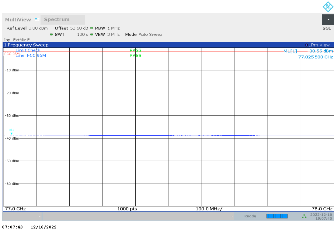
Plot no. 70: radiated emissions 77 GHz – 78 GHz, BEC high, f_{low} , Mode 1, polarization aligned with radar sensor
