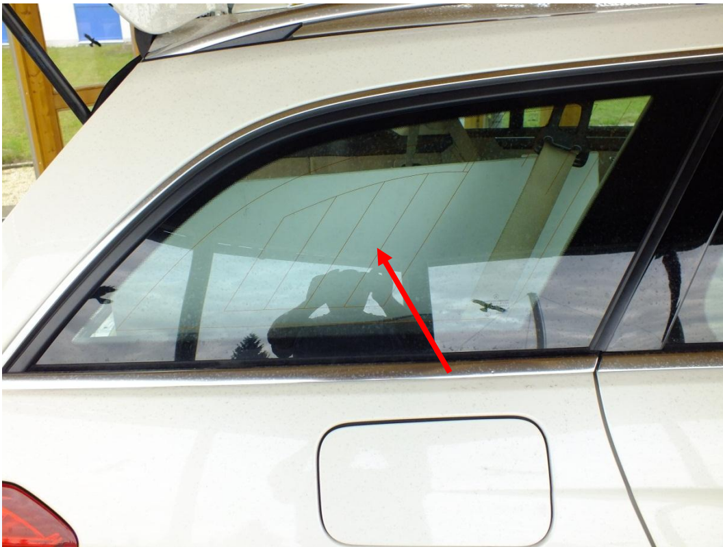
UT connected to the dedicated window antenna in the original integration of a car.
