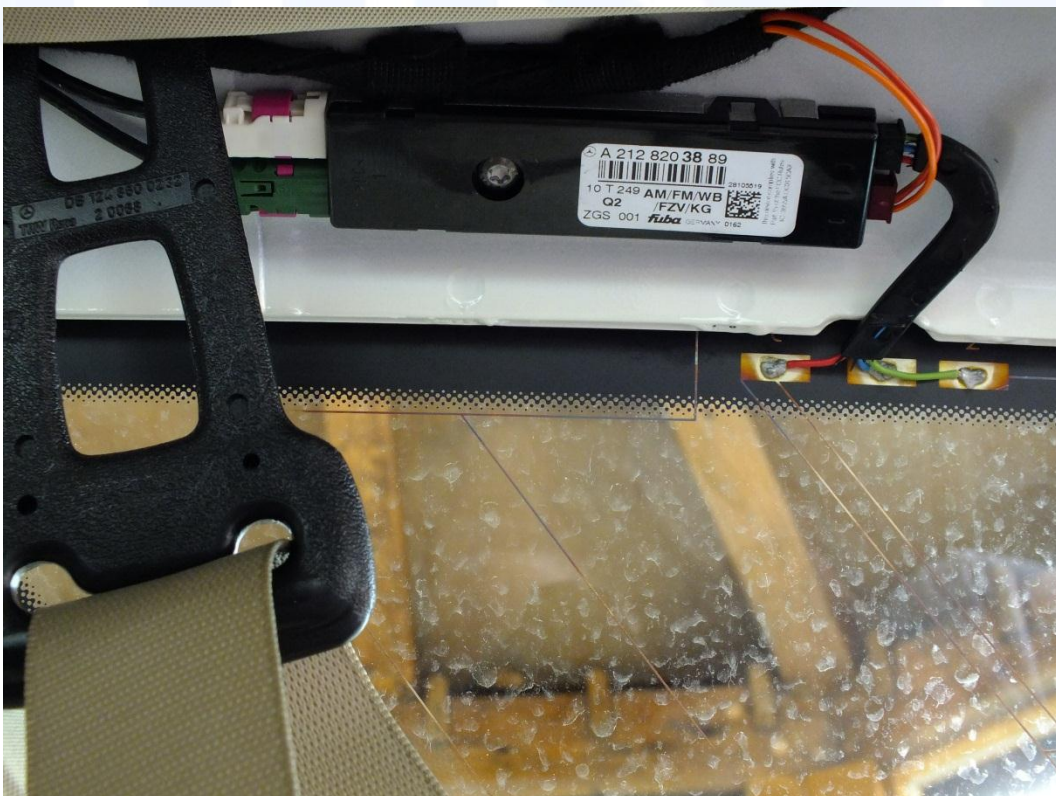
UT connected to the dedicated window antenna in the original integration of a car.
