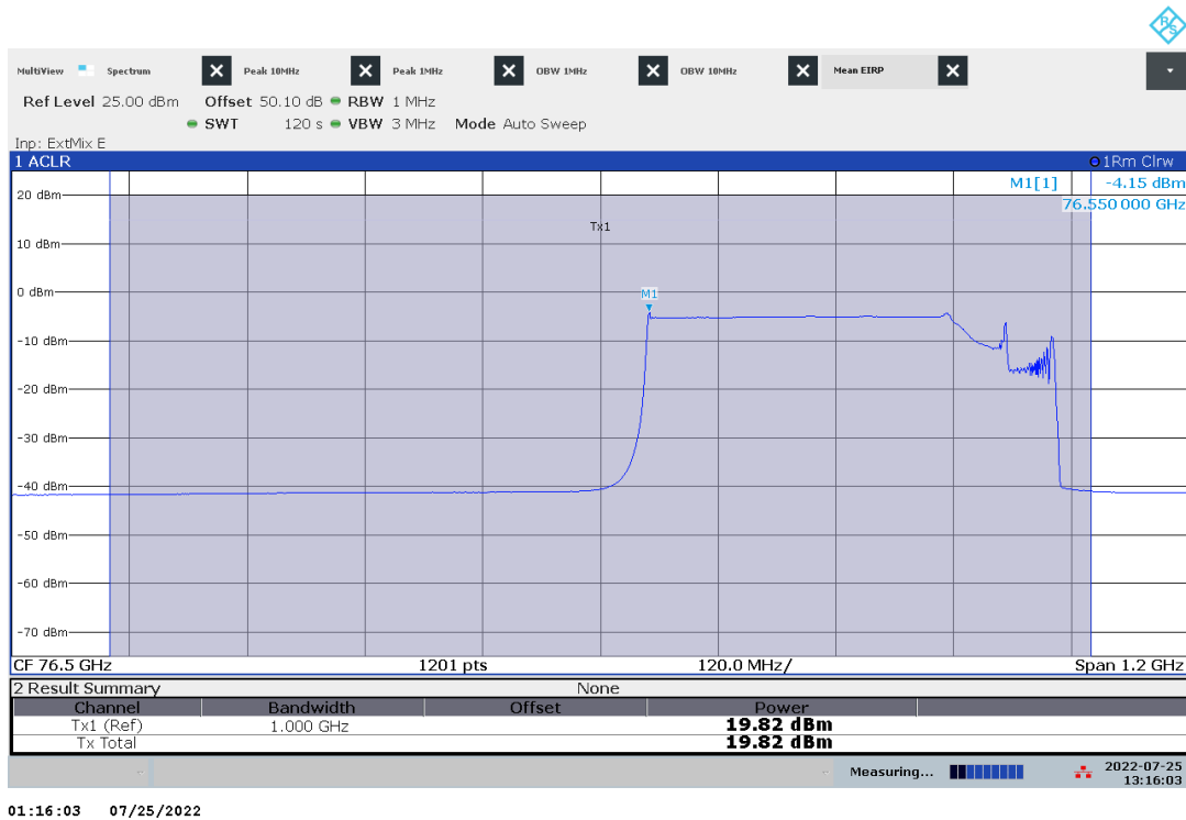
Plot no. 6: Mean Power EIRP, RMS detector / Channel Power, Mode 2, f_{high} , T_{nom}
