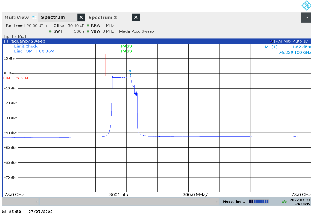
Plot no. 41: radiated emissions 75 GHz – 78 GHz, BEC, f_{low} , Mode 1, polarization aligned with radar sensor
