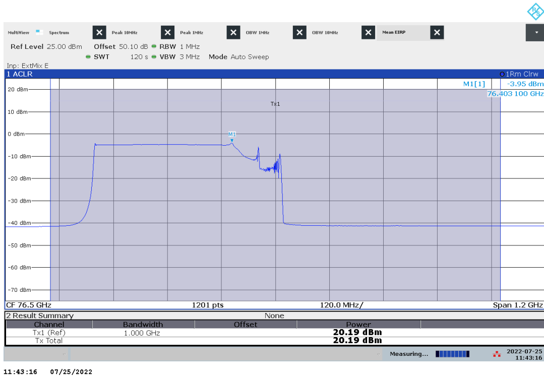
Plot no. 4: Mean Power EIRP, RMS detector / Channel Power, Mode 2, f_{low} , T_{nom}
