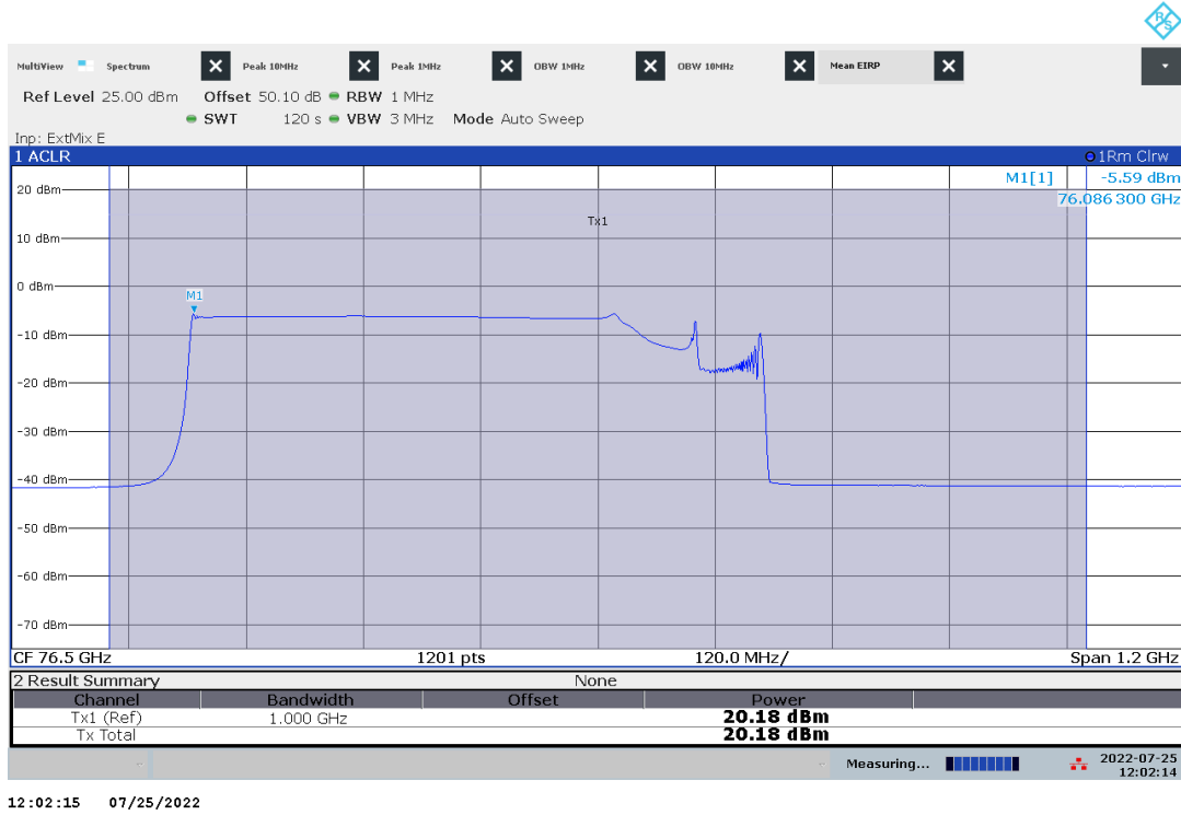
Plot no. 7: Mean Power EIRP, RMS detector / Channel Power, Mode 3, f low , T nom
