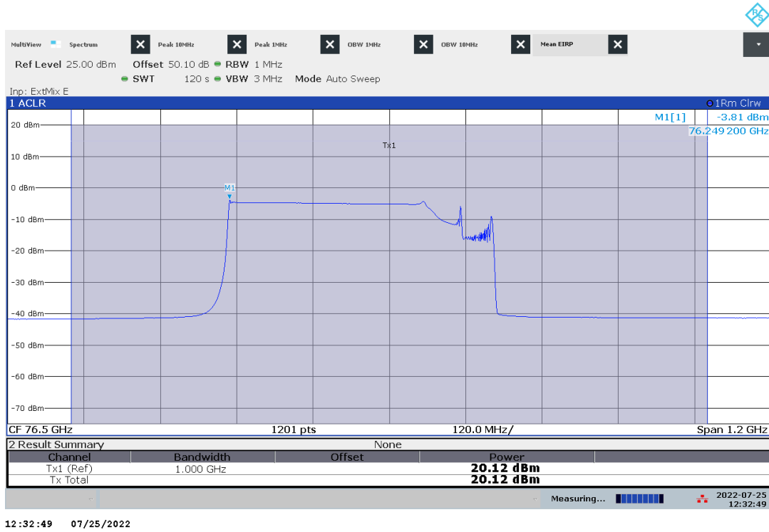
Plot no. 5: Mean Power EIRP, RMS detector / Channel Power, Mode 2, f_{mid} , T_{nom}
