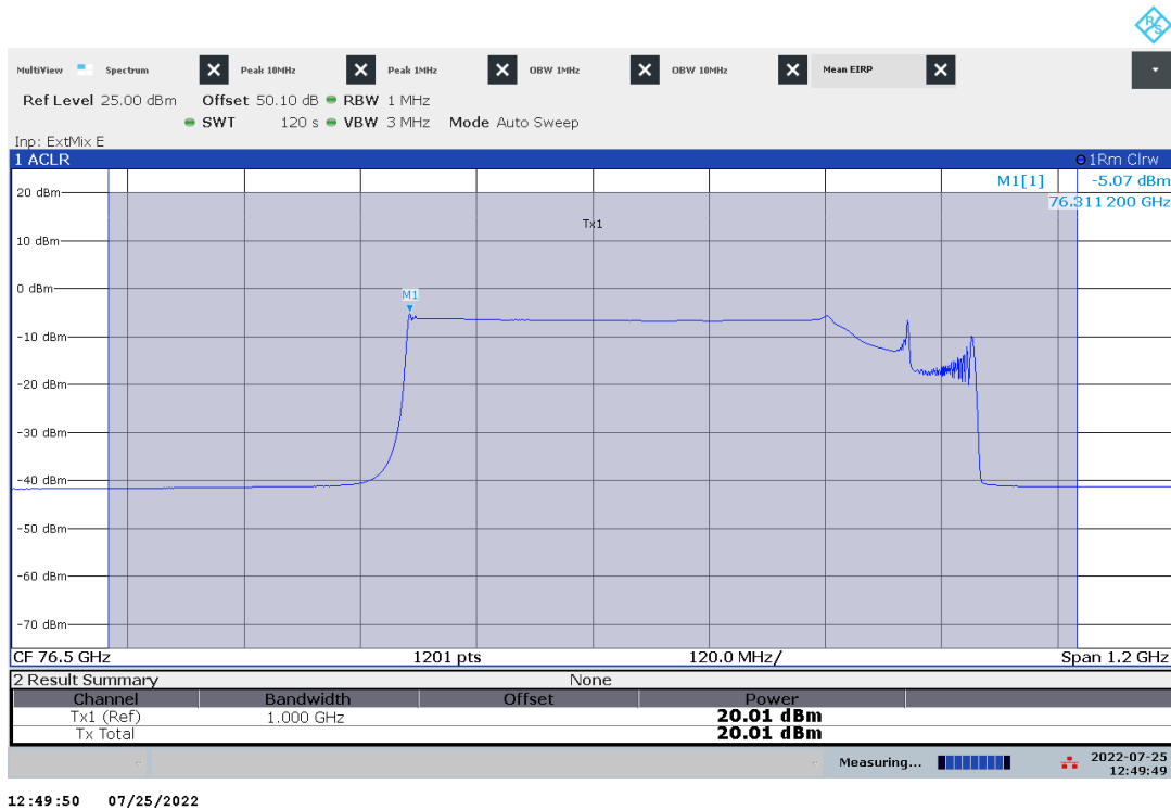
Plot no. 8: Mean Power EIRP, RMS detector / Channel Power, Mode 3, f mid , T nom
