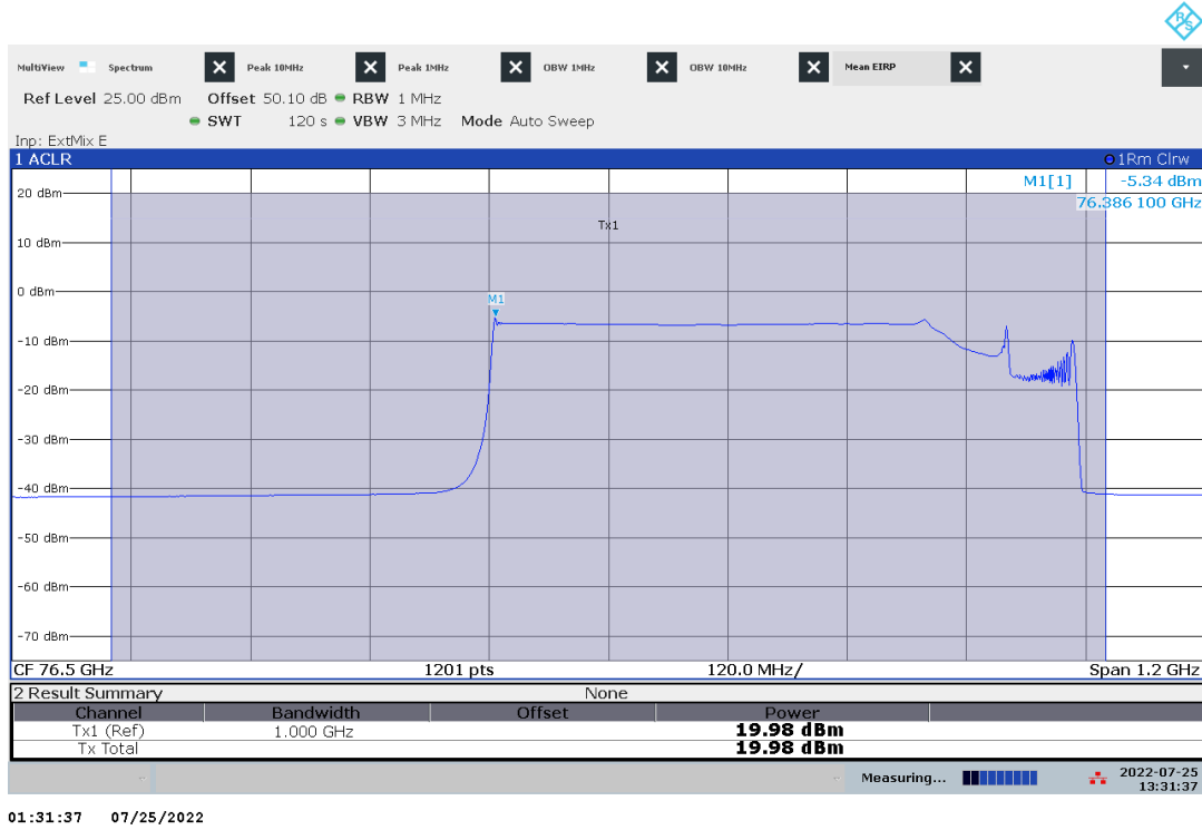
Plot no. 9: Mean Power EIRP, RMS detector / Channel Power, Mode 3, f_{high} , T_{nom}
