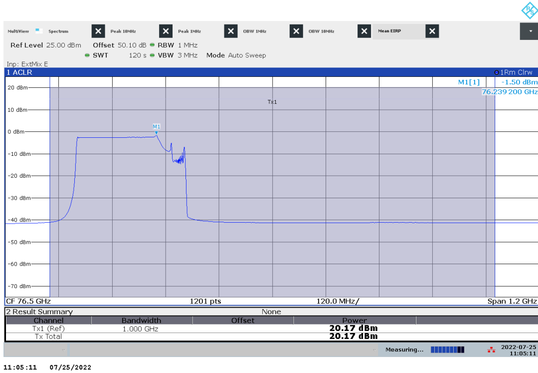
Plot no. 1: Mean Power EIRP, RMS detector / Channel Power, Mode 1, f low , T nom
