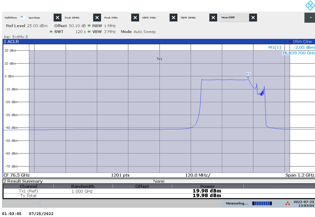
Plot no. 3: Mean Power EIRP, RMS detector / Channel Power, Mode 1, f_{high} , T_{nom}
