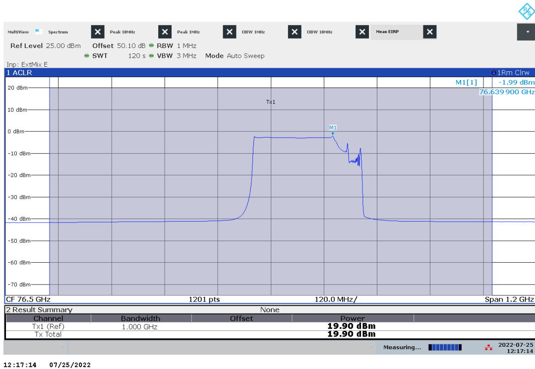
Plot no. 2: Mean Power EIRP, RMS detector / Channel Power, Mode 1, f mid , T nom
