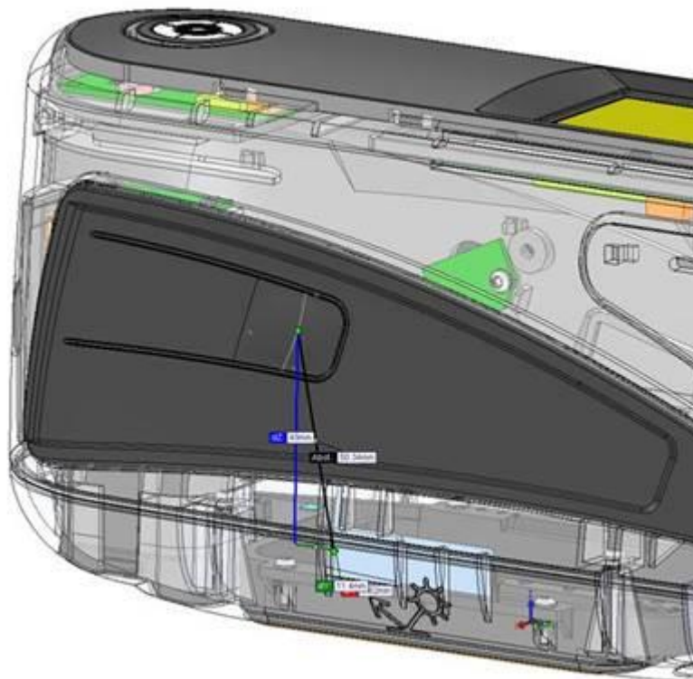
Antenna to thumb button distance 50.34 mm
