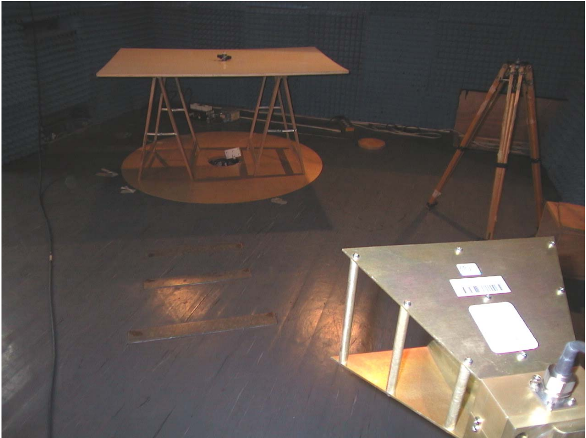
Photo-3 Radiated Emission 1GHz – 18GHz
