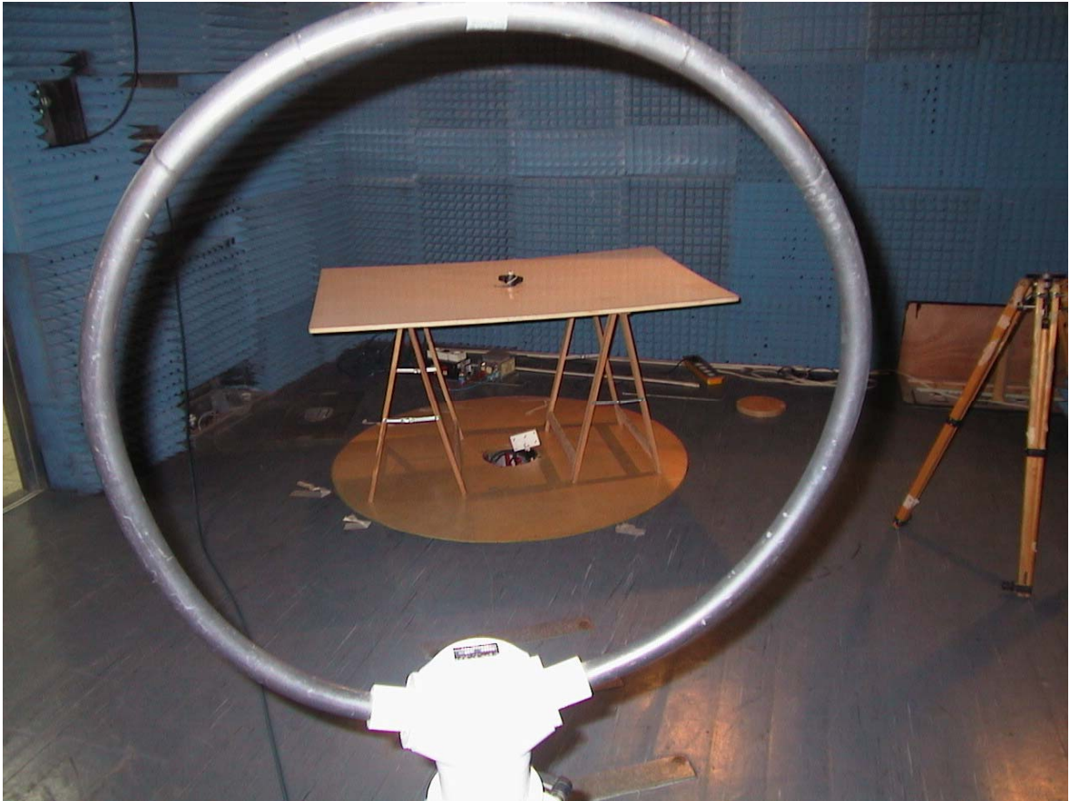
Photo-1 Radiated Emission up to 30MHz
