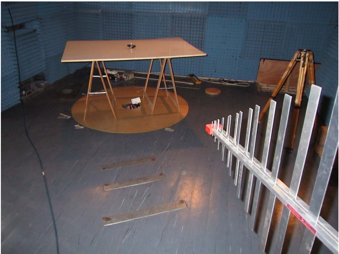
Photo-2 Radiated Emission 30MHz – 1GHz
