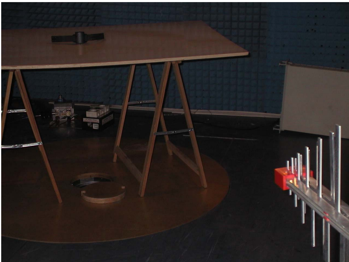
Radiated Emission Test Setup 30MHz-1GHz
