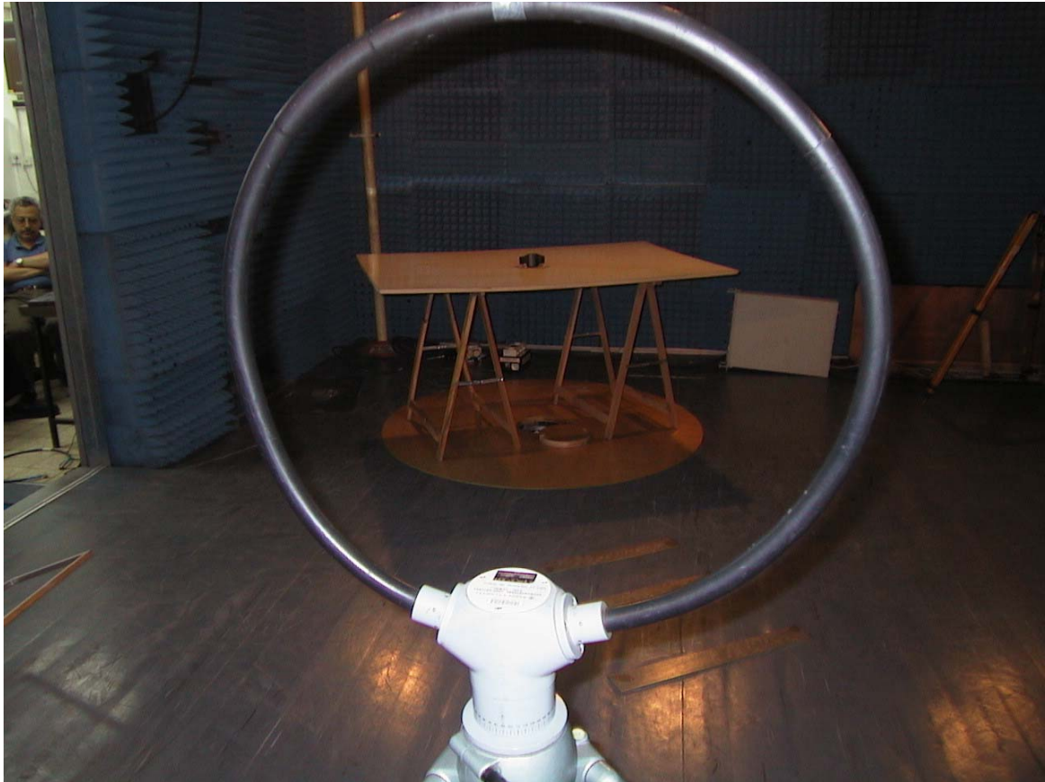
Radiated Emission Test Setup up to 30MHz
