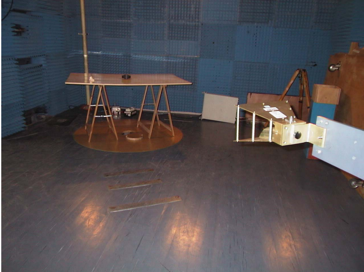
Radiated Emission Test Setup 1GHz-18GHz
