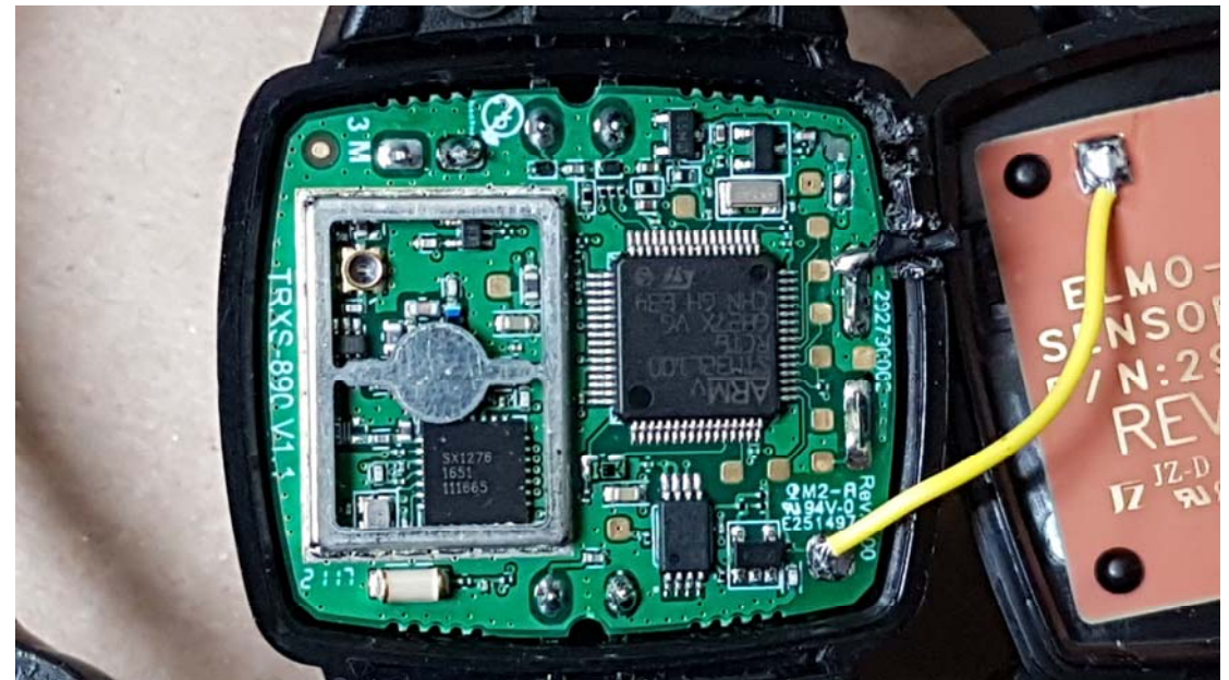
RF module with removed shielding
