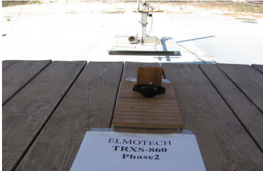
Figure 2. Radiated Emission Test Above 1 GHz
