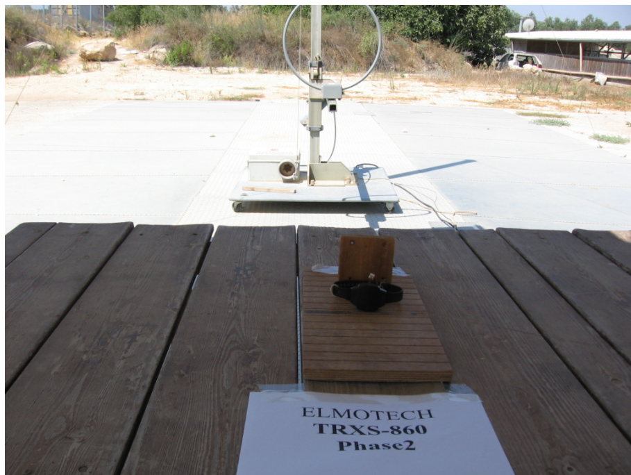
Figure 3. Radiated Emission Test 9 kHz – 30 MHz
