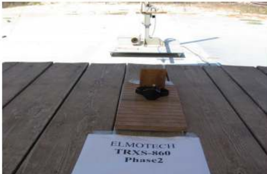
Figure 2. Radiated Emission Test Above 1 GHz
