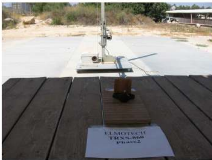
Figure 4. Radiated Emission Test 30 MHz – 1000 MHz
