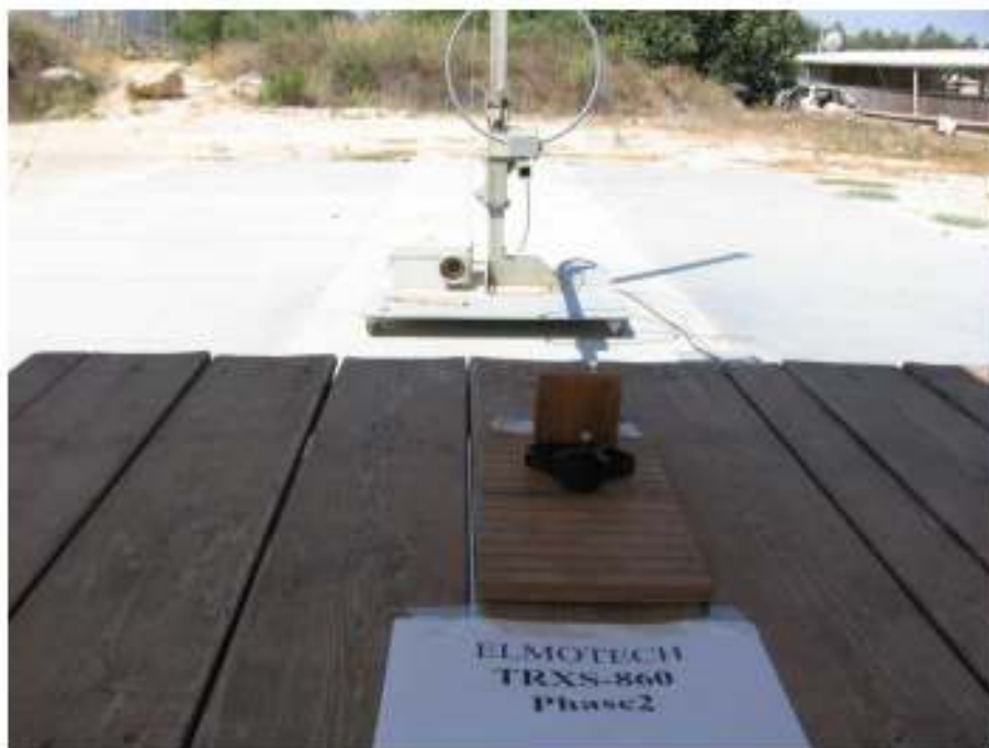
Figure 3. Radiated Emission Test 9 kHz – 30 MHz
