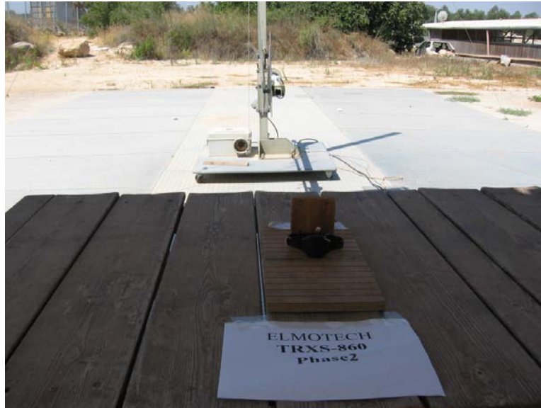
Figure 2. Radiated Emission Test 30 MHz – 1000 MHz
