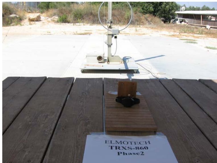
Figure 3. Radiated Emission Test 9 kHz – 30 MHz
