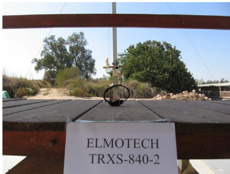
Figure 2. Radiated Emission Test 9 kHz – 30 MHz
