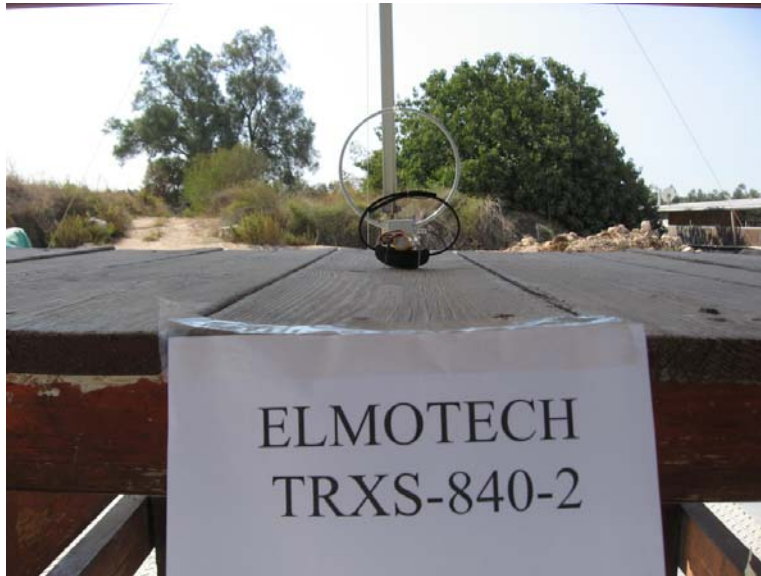
Figure 2. Radiated Emission Test 9 kHz – 30 MHz
