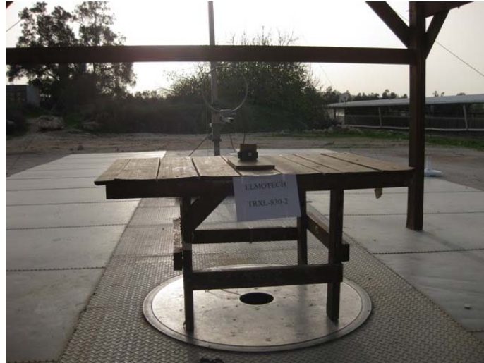
Figure 2. Radiated Emission Test 9 kHz – 30 MHz
