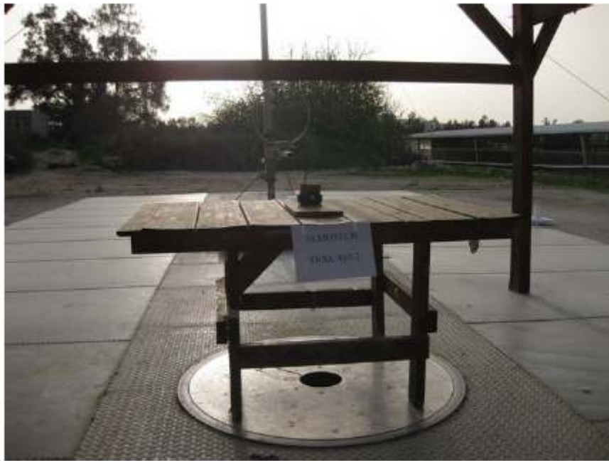
Figure 2. Radiated Emission Test 9 kHz – 30 MHz
