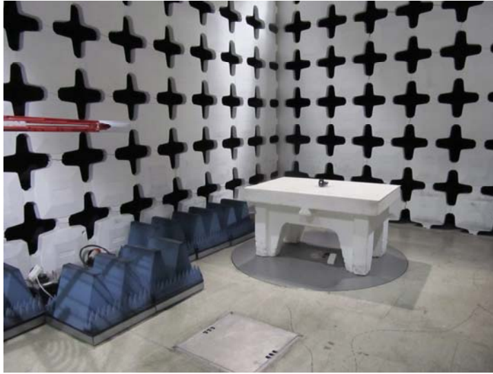
Radiated emissions test set up below 1GHz.
