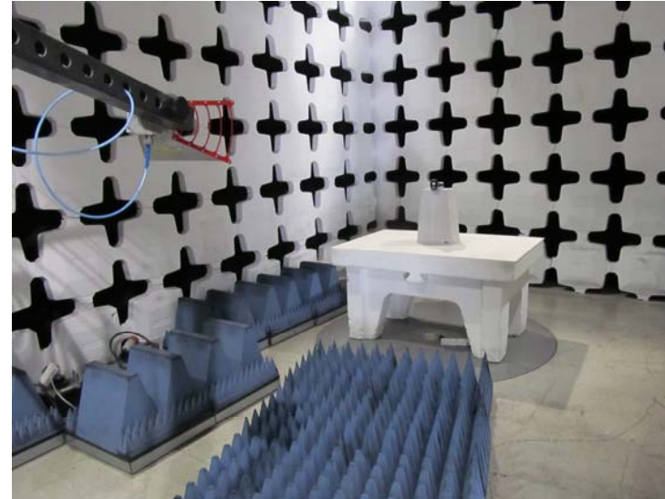
Radiated emissions test set up above 1GHz.
