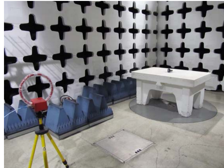
Radiated emissions test set up below 30MHz.
