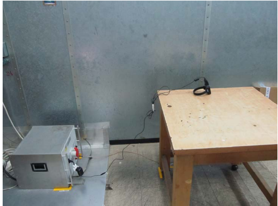
Conducted emissions test set up.
