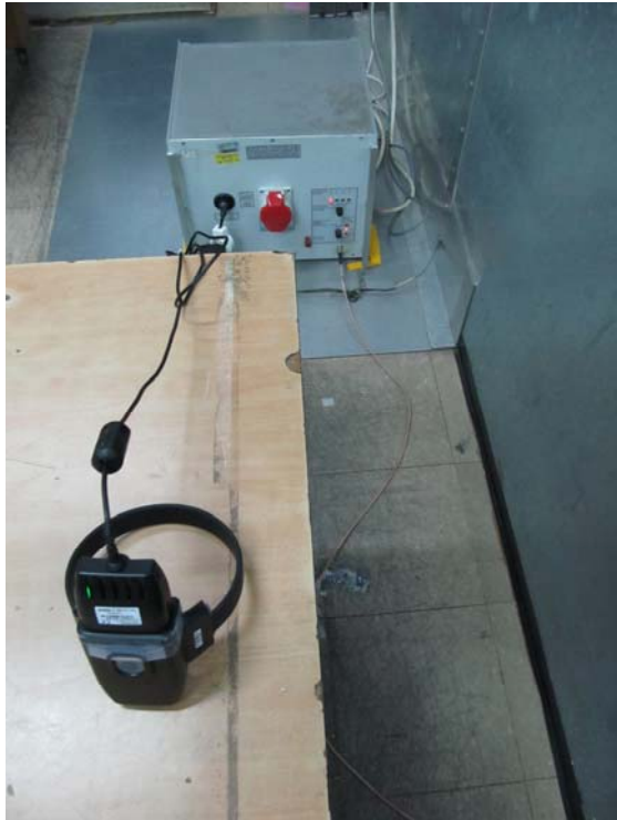
Conducted emissions test set up.
