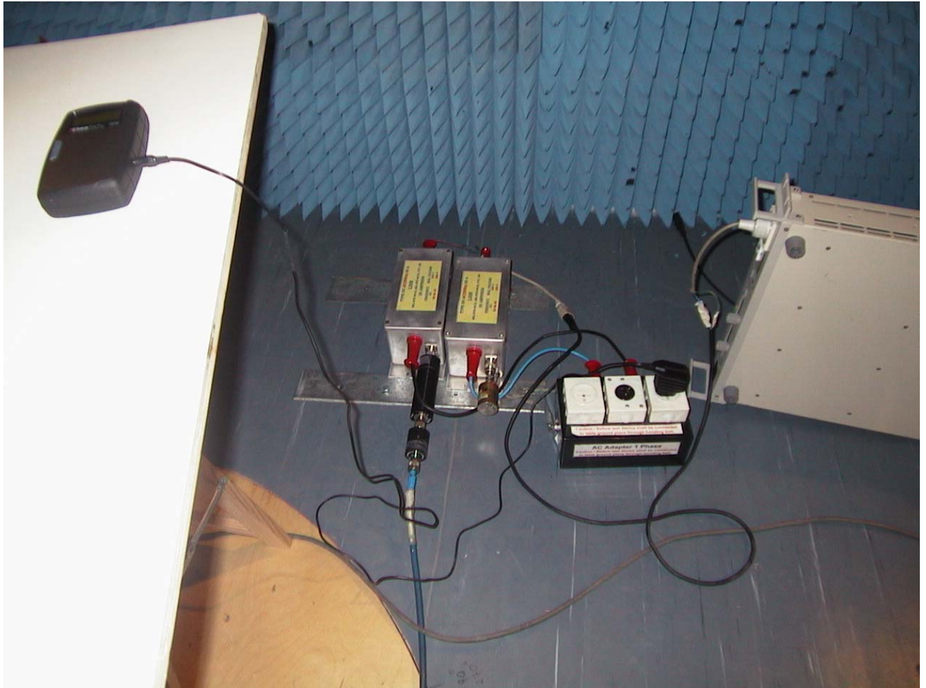
Picture CE/1 Conducted Emission Setup
