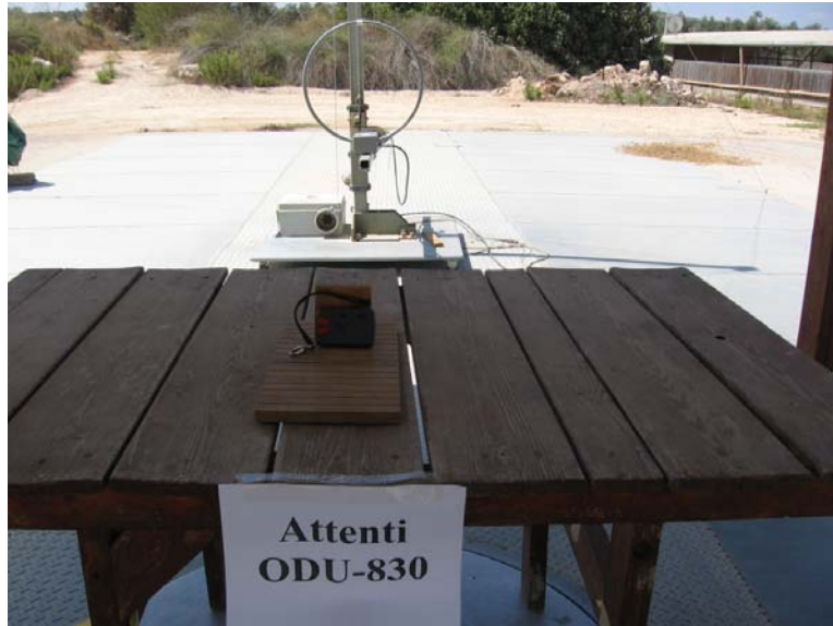
Figure 2. Radiated Emission Test 9 kHz – 30 MHz
