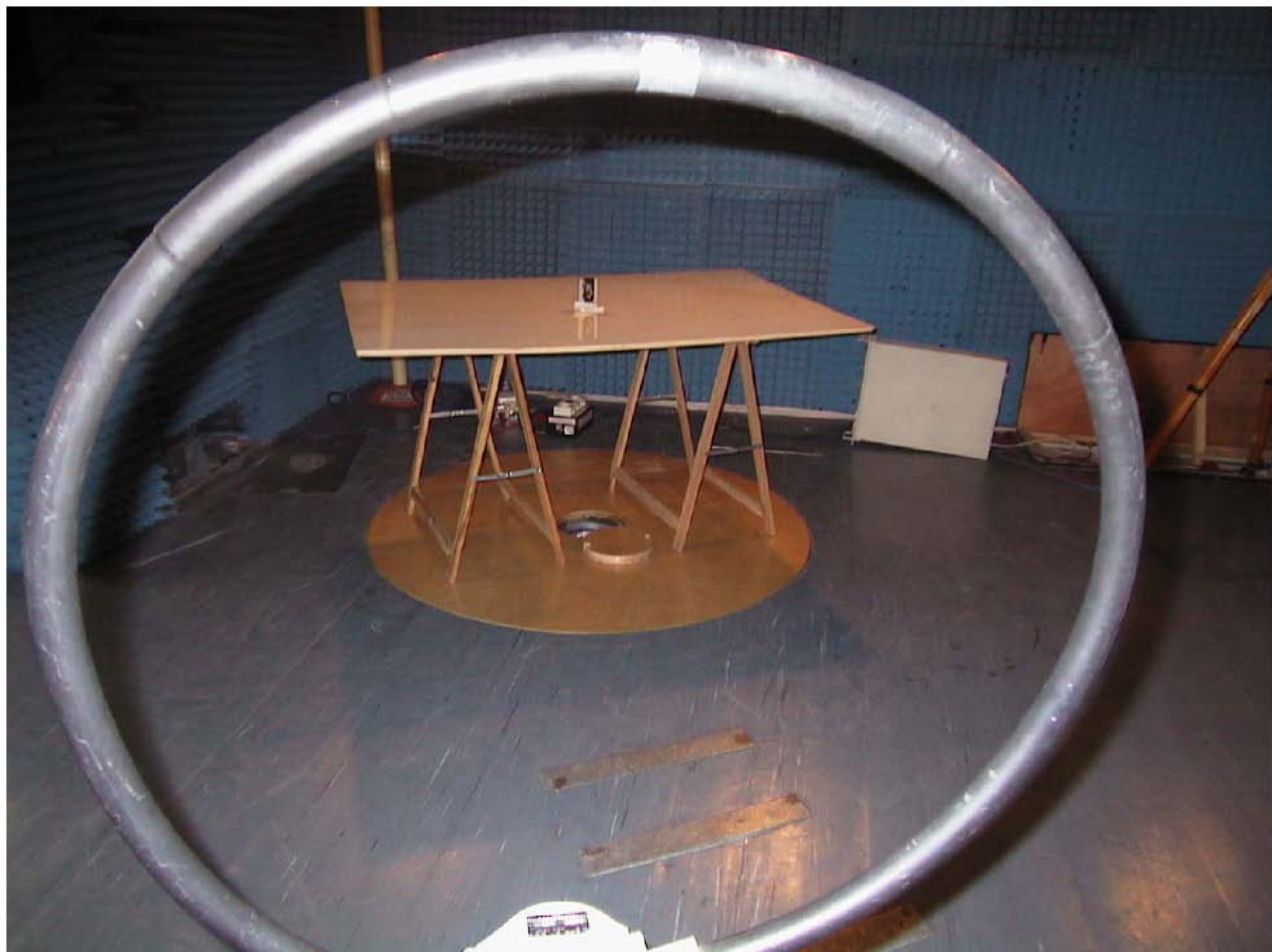
Photograph-2 Set up for Radiated Emission up to 30MHz
