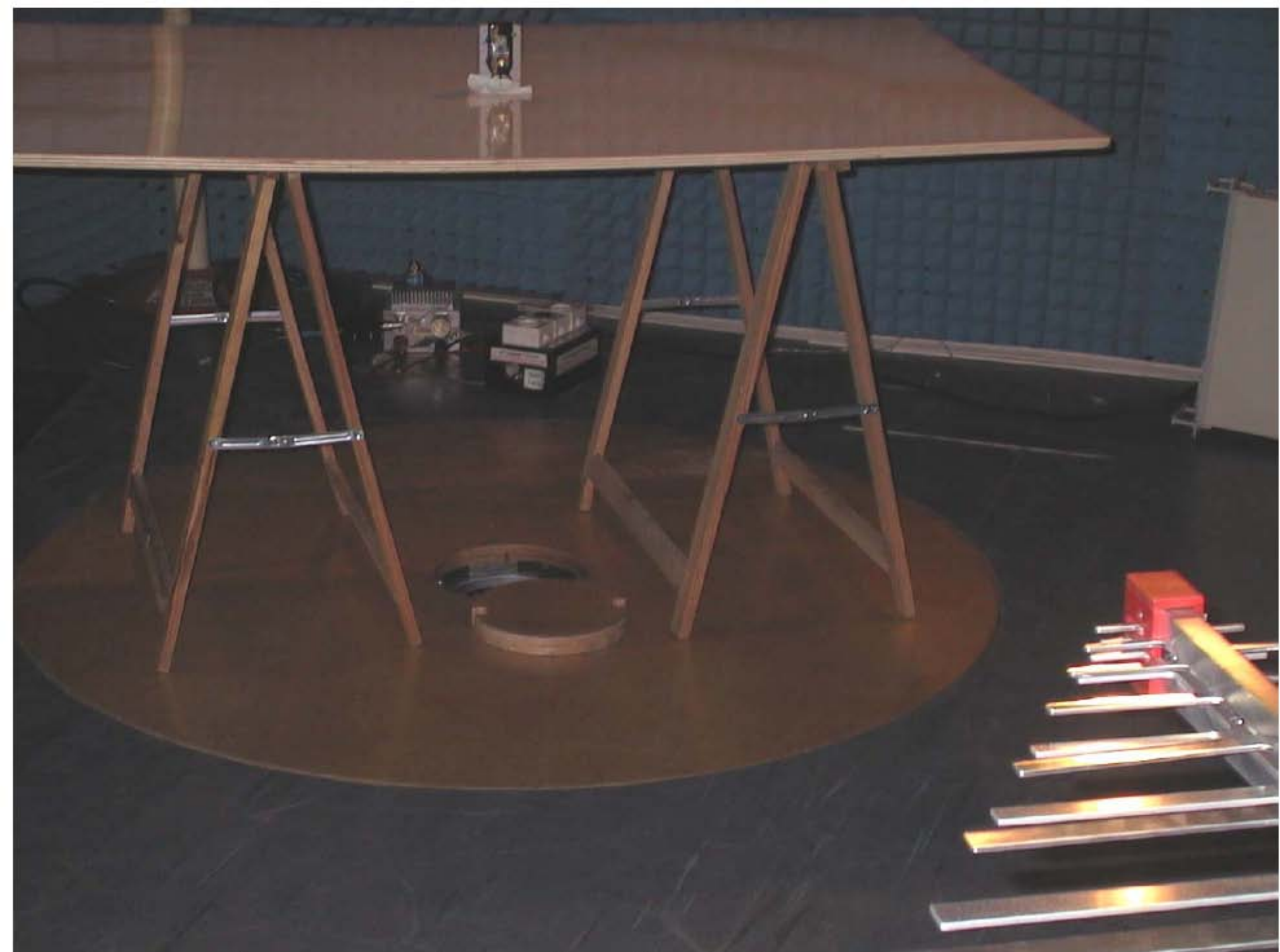
Photograph-3 Set up for Radiated Emission 30MHz-1GHz
