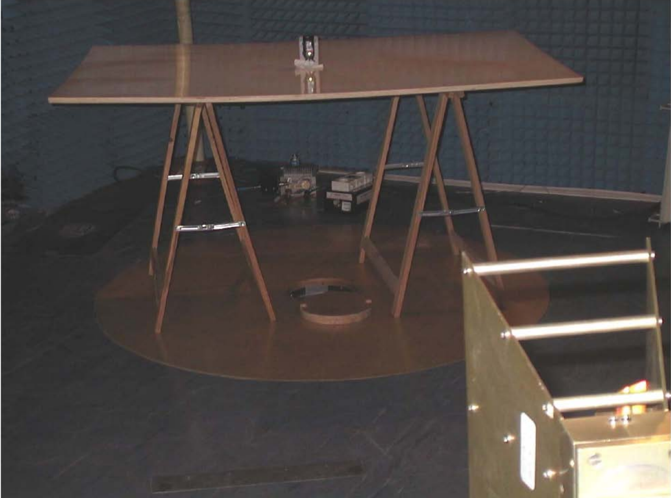
Photograph-4 Set up for Radiated Emission 1GHz-5GHz
