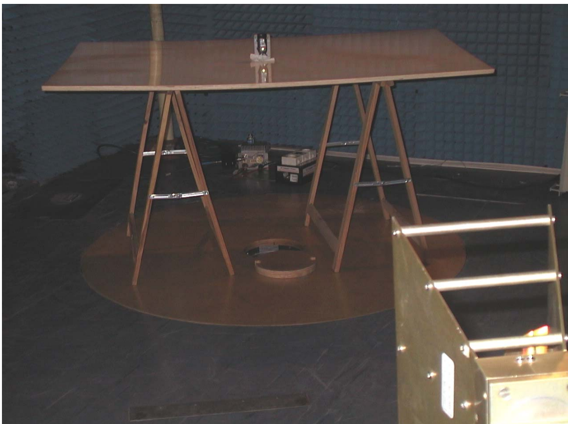
Photograph-4 Set up for Radiated Emission 1GHz-5GHz
