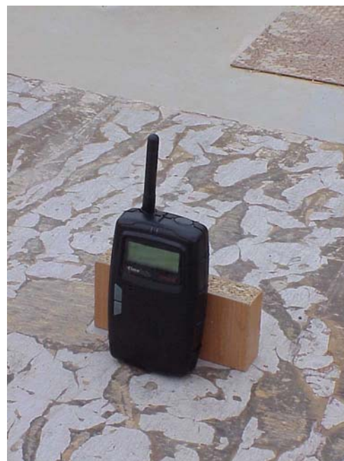
Photo 3. Emissions test setup on OATS. Receive mode.
