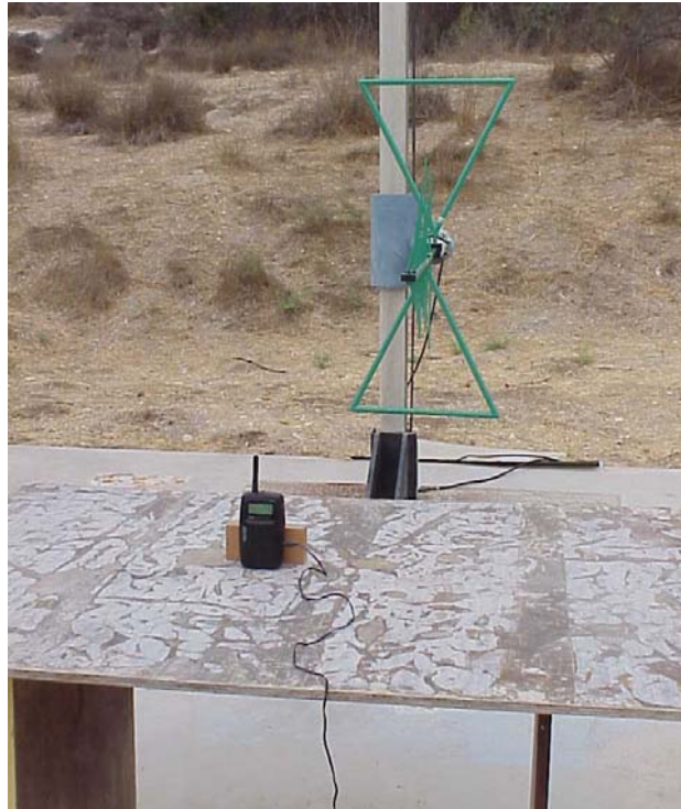
Photo 2. Emissions test setup on OATS. Charge mode.
