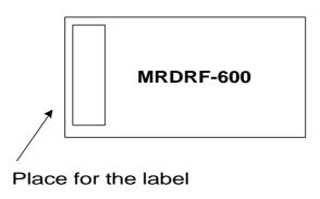
The compliance statement (pursuant to sect. 15.19 (a) (3)) must be labeled on the device but due to the small dimensions of MRDRF-600 this statement is inserted in the User manual only (refer to p. 7 of the User manual).
