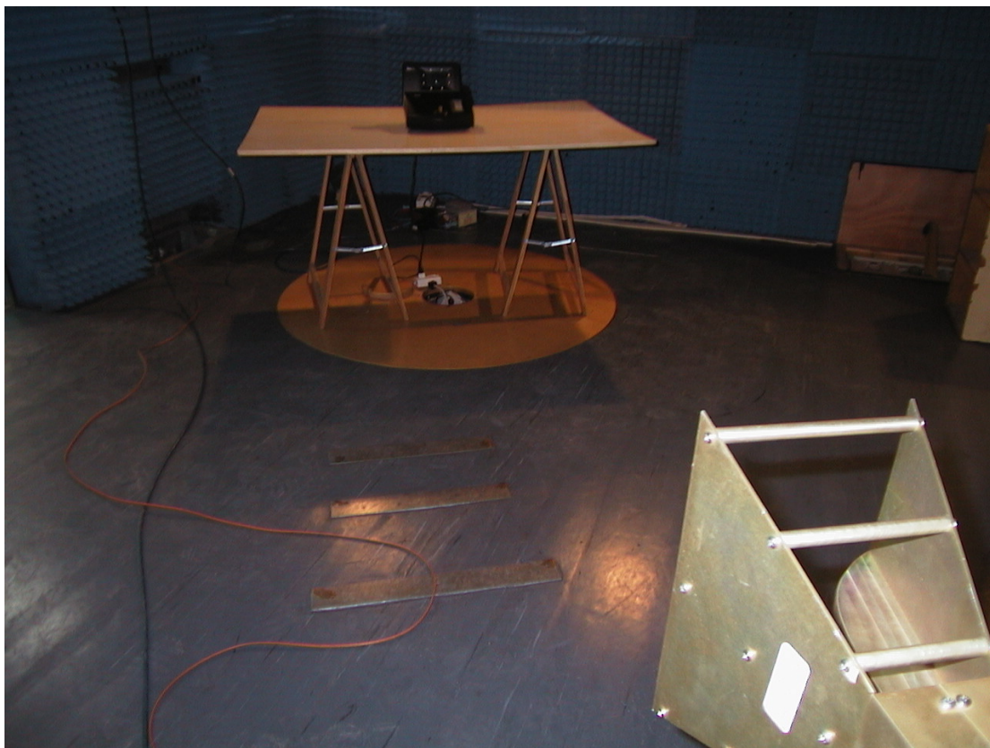
Photograph/ 2 Radiated Emission 1-2GHz test setup
