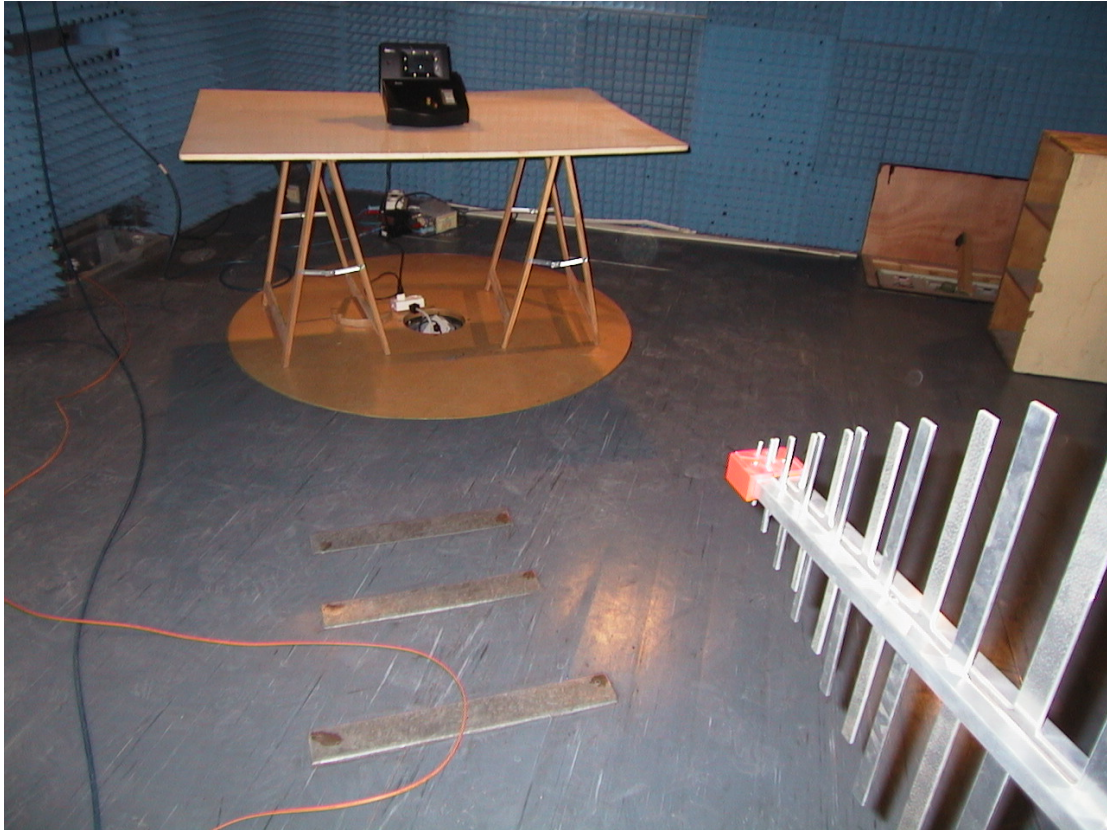
Photograph/ 1 Radiated Emission 30-1000MHz test setup
