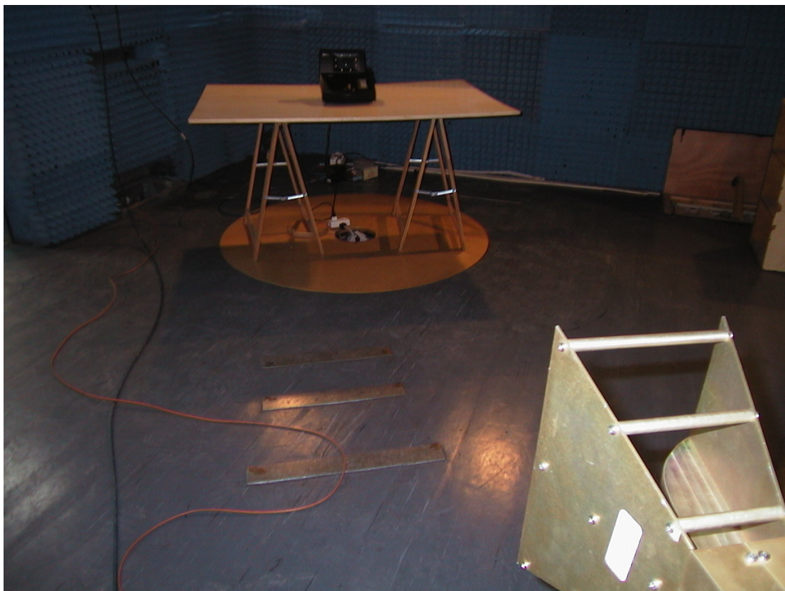
Photograph/ 2 Radiated Emission 1-2GHz test setup
